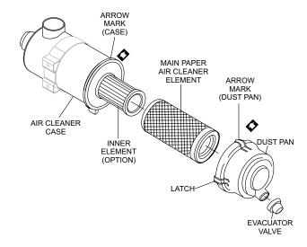
Figure 19. Air Cleaner Components
